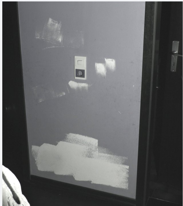
Repaintings / overcoatings on wall, standard light, UV-reflection - Copyright Dr. M. Schulz, Institute of Legal Medicine LMU Munich
